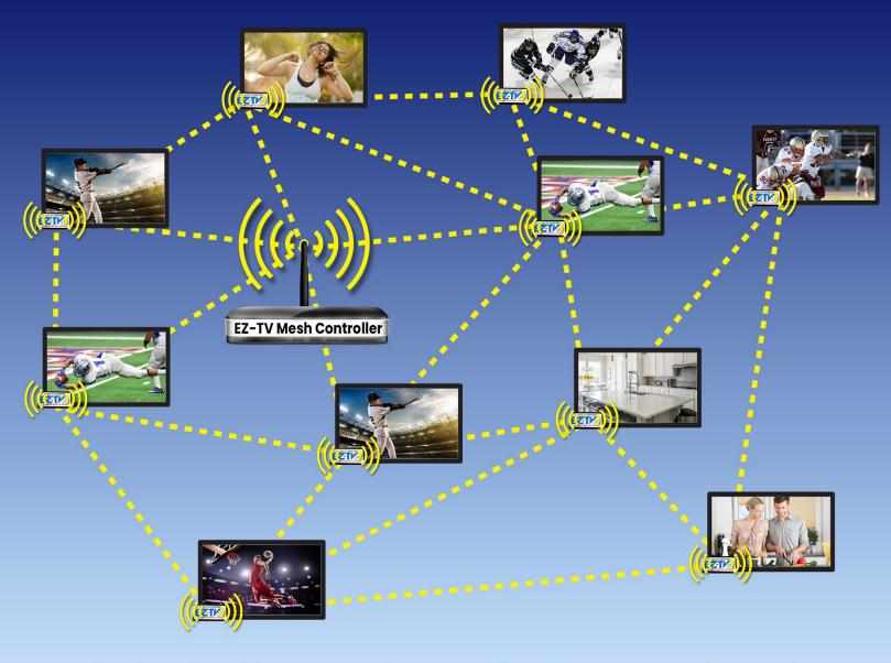
Simply put, a Mesh network uses radios that communicate with each other to pass information from radio to radio until it gets to it's destination. This kind of system allows for very large installations as commands hop from one EZ-TV TV module to the next with a range of 50 feet between TV's we can cover the largest of venues!
